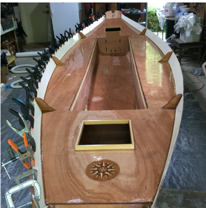
Photo 6: Decking complete with hatches and a bit of decorative marquetry at the bow end.
