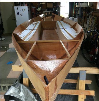
Photo 5: Interior showing frames, stringers and foam flotation.
