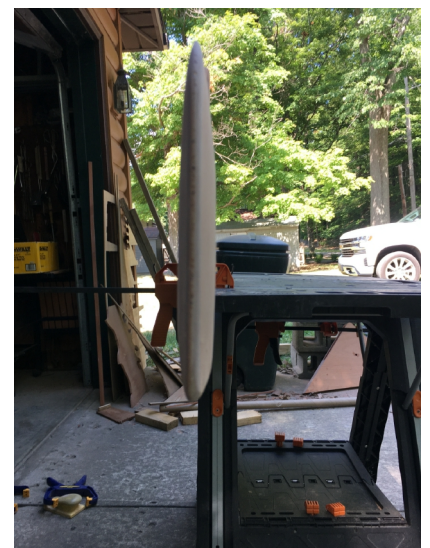
Photo 10: The centerboard faired fore and aft.
